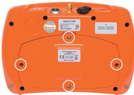
Fig. 40: Back of the C 200 receiver White circles: Screws of battery compartment cover
