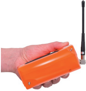
Fig. 6: Receiver in its normal position of use The aerial is pointing upwards.
